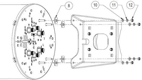
3. Connect item3 to above sub-assembly by M12 screw, washer and nut (No need to tight).
