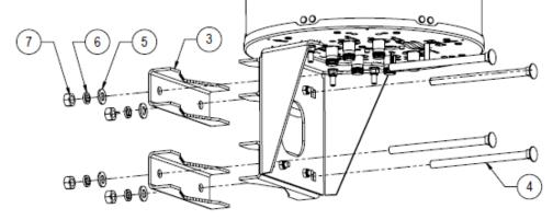
4. Insert the full assembly to pole and tight M12 nut with 40 Nm / 30 ft-lbs torque.
